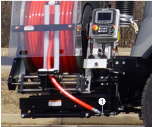
Winter Recirculation Fitting
