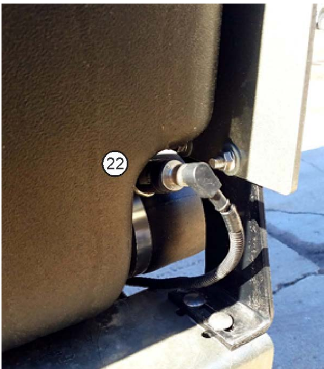
Figure 5-13: Fresh Water Tank Level Sensor
