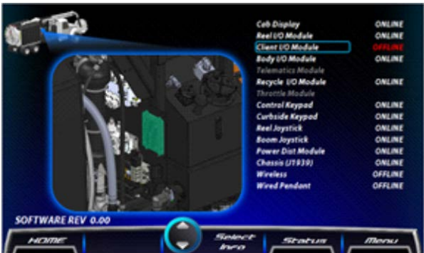
Control System Status
