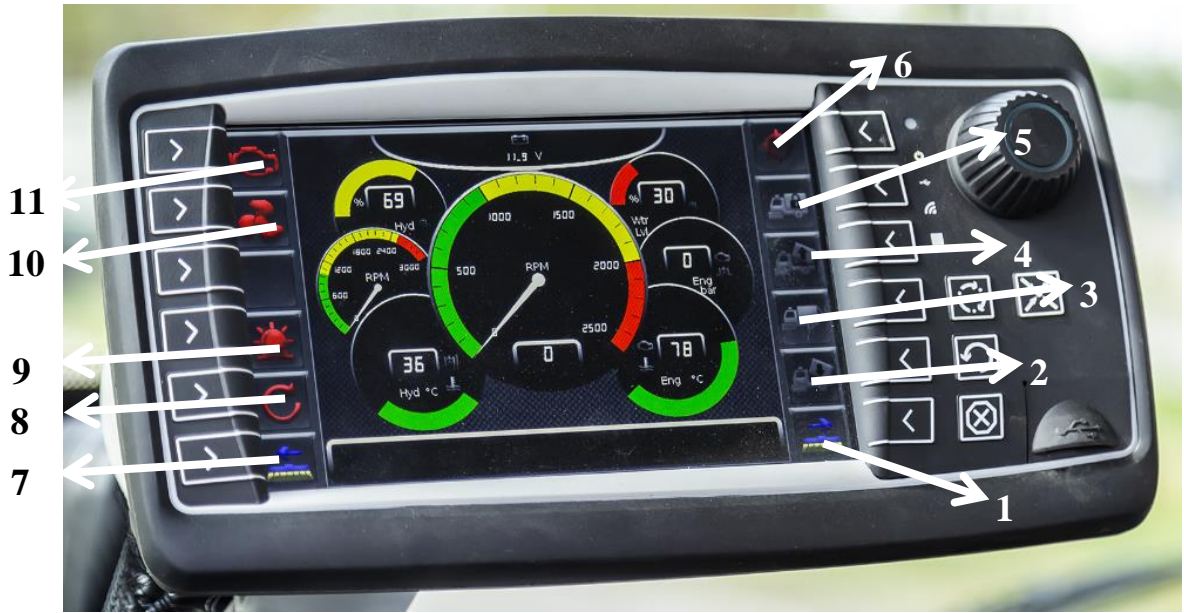
Figure 4.5: Touch Control Panel
